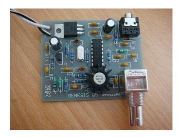
Current consumption is approx. 110mA @12.8V. (approx. 130 mA key down). Should you wish to increase output power replace R7 with 220R. Under normal operation condition 2N3866 will get fairly hot - even while not transmitting. However this is quite acceptable - 2N2866 is robust transistor capable of 3W dissipation at 200C.
