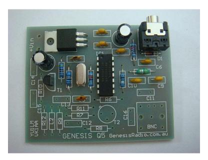
After the assembly of the oscillator, connect the input voltage and keyer. Current consumption is approx. 40mA @12.8V. You should be able to hear Q5 oscillator on your receiver.
